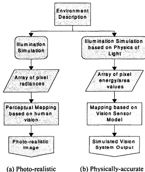
Figure 9 Model of the synthetic imaging process
