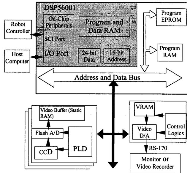
Figure 6 Schematic of a flexible integrated vision system
